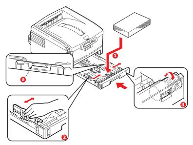
**4.** Adjust the rear stopper and paper guides (2) to the size of paper being used. For A6 paper, remove and re-install in the A6 position.
